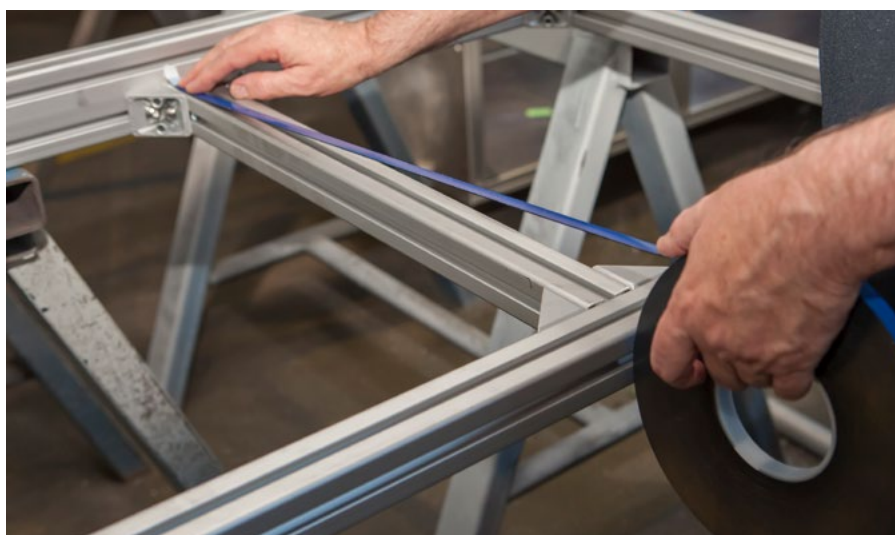
tesa® ACX plus 7048 mounting panel to subframe
